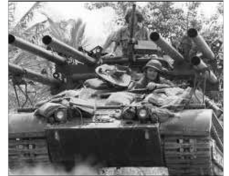
The Ontos proved to be a perfect "shoot and scoot" weapon in Hue City where it could pull out from behind a building, shoot a devastating salvo of its 106 mm recoilless rifles at the enemy, and then scoot back around the corner for cover.
